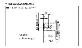
1) ANSI B92.1a, 30° pressure angle, flat root, side fit, tolerance class 5
