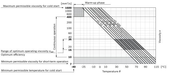
1) At temperatures below -25 °C, an NBR shaft seal is required (permissible temperature range -40 °C bis +90 °C)
