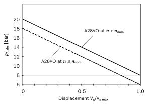
▼ Maximum permissible rotational speed (rotational speed limit) (p<sub>s abs</sub> = inlet pressure [bar])
