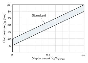
Pilot pressure increase  $V_{\rm g\;min}$  to  $V_{\rm g\;max}$ :  $\Delta p$  = 25 bar When ordering, state in plain text:
