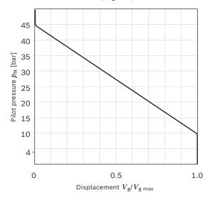
Pilot pressure increase  $V_{\rm g\ max}$  to  $V_{\rm g\ min}$ :  $\Delta p$  = 35 bar
