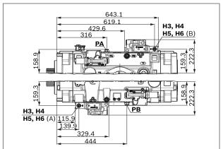
▼ D2 - pressure control, electric-proportional with integrated pilot valve for external pilot pressure supply
