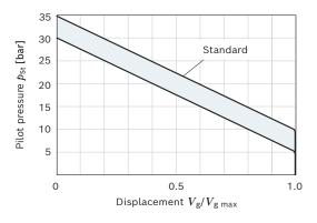
Pilot pressure increase  $V_{\rm g \; max}$  to  $V_{\rm g \; min}$ :  $\Delta p$  = 25 bar When ordering, state in plain text:
