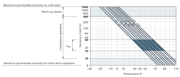
$<sup>^{1)}</sup>$  This corresponds, for example on the VG 46, to a temperature range of +4  $^{\circ}\text{C}$  to +85  $^{\circ}\text{C}$  (see selection diagram)
