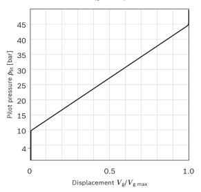
Pilot pressure increase  $V_{\rm g\;min}$  to  $V_{\rm g\;max}$ :  $\Delta p$  = 35 bar
