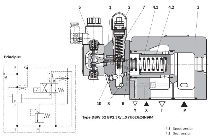
With version "DBW  $\dots Y \dots$ ", the connection T-Y is closed.
