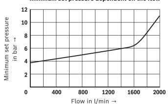
1) The characteristic curves apply for output pressure  $p_T = 0$  bar in the entire flow range
