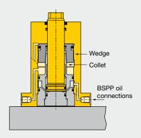
Hydraulic pressure pushes the collet up a wedge, locking the plunger in the clamping position.
